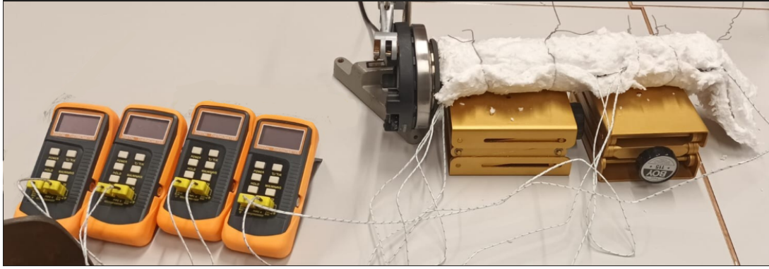
Figure 3: Photograph of the experimental setup used to measure heat propagation along the aluminium rod. [Author's Own]
