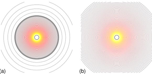
**Comparison** of field around a live wire with and without shielding by a conducting sheet.
